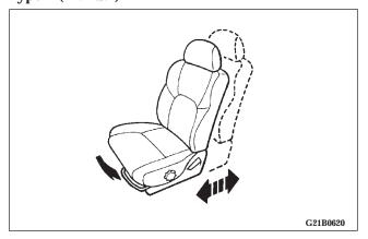
Pull the seat adjusting lever and slide the seat forward or backward to the desired position. Release the adjusting lever to lock the seat in position.
